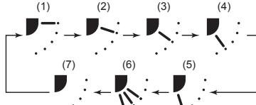
\* When cooling or drying, (4) and (5) are not displayed.
