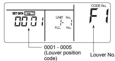
\* F1 appears in the CODE No. section on the remote controller. This indicates that the louver 01 shown in the following figure is selected.
